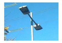
Below: Typical well directed full cut-off street lighting, with shields.
